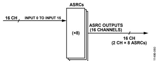
Figure 57. Example ASRC Routing, Bypassing DSP Core
