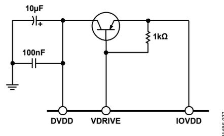
Figure 24. External Components Required for Voltage Regulator Circuit
