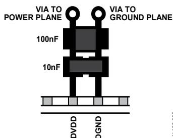
Figure 82. Layout for Multiple Power Supply Bypass Capacitors
