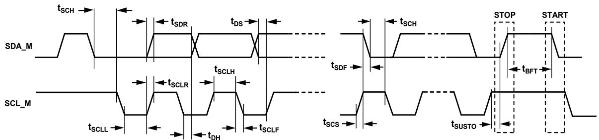
Figure 8. I<sup>2</sup>C Master Port Timing Specifications
