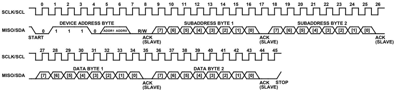
Figure 28. I<sup>2</sup>C Slave Single Word Write Operation (Two Bytes)
