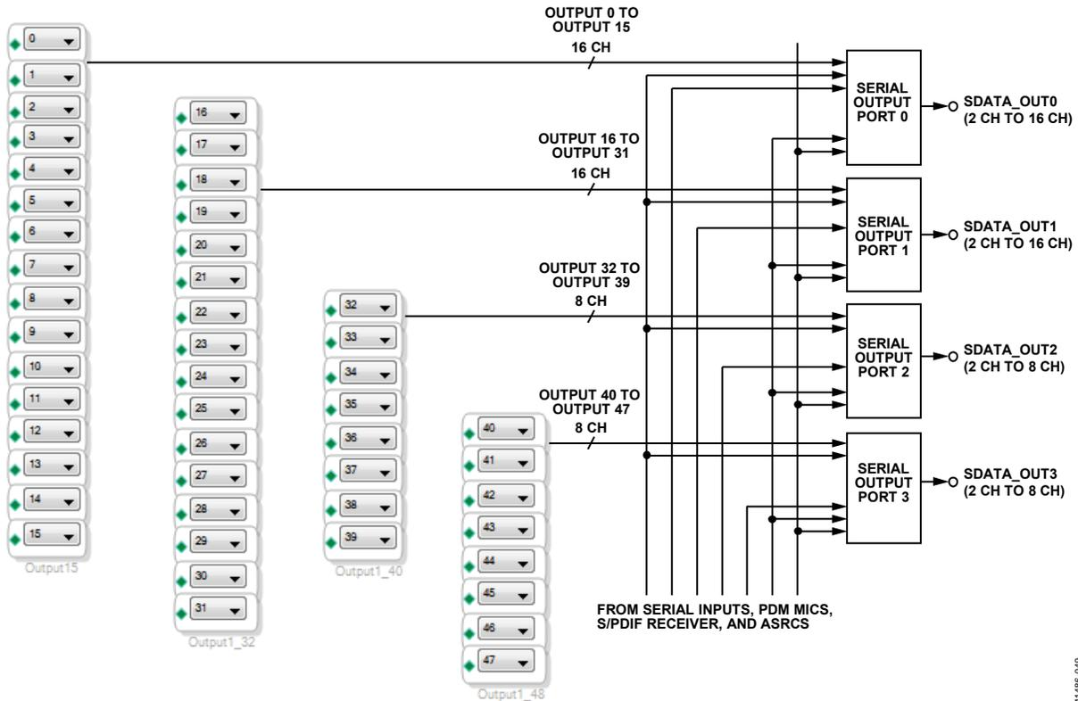
Figure 46. DSP to Serial Output Mapping in SigmaStudio
