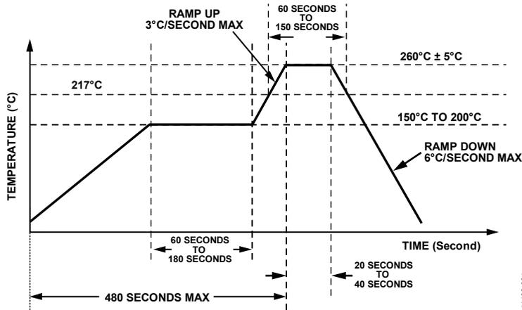
Figure 89. Soldering Profile
