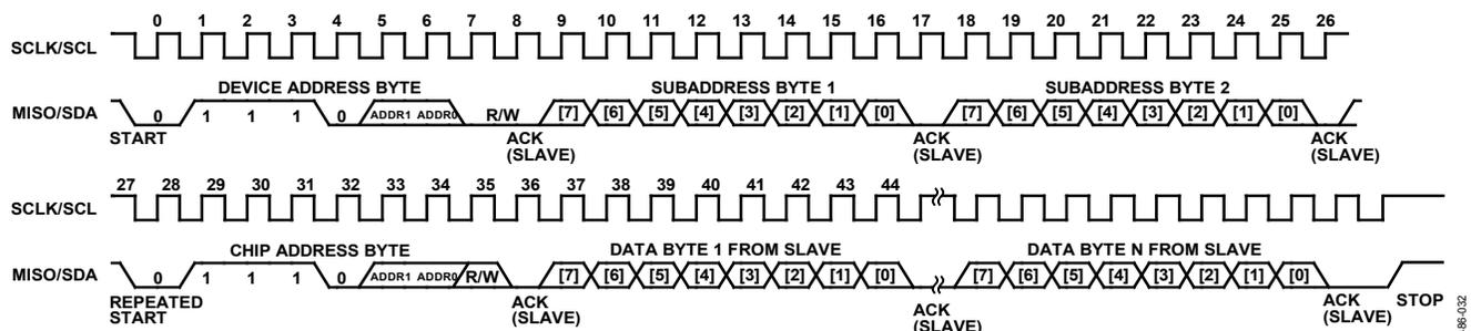
Figure 30. I<sup>2</sup>C Slave Burst Mode Read Operation (N Bytes)
