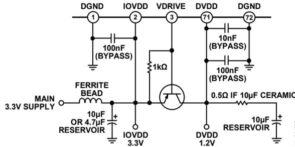
Figure 86. Ferrite Bead Power Supply Isolation Circuit Example
