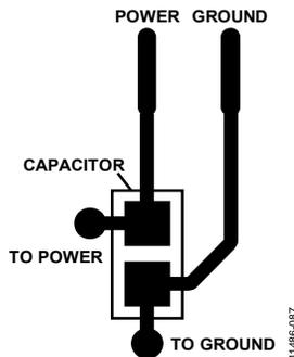
Figure 81. Recommended Power Supply Bypass Capacitor Layout
