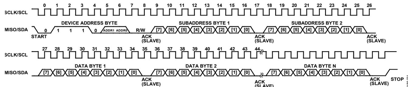
Figure 29. I<sup>2</sup>C Slave Burst Mode Write Operation (N Bytes)
