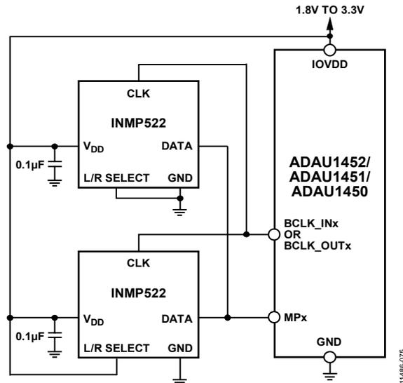
Figure 72. Example Stereo PDM Microphone Input Circuit
