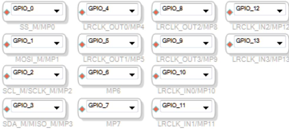
Figure 76. Complete Set of General-Purpose Outputs in SigmaStudio
