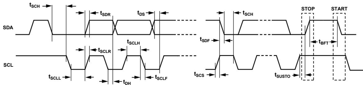
Figure 7. I<sup>2</sup>C Slave Port Timing Specifications
