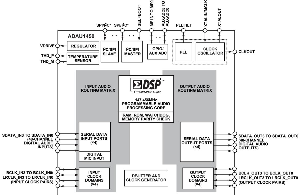
\*SPI/I<sup>2</sup>C INCLUDES THE FOLLOWING PIN FUNCTIONS: SS\_M, MOSI\_M, SCL\_M, SCLK\_M, SDA\_M, MISO\_M, MISO, SDA, SCLK, SCL, MOSI, ADDR1, SS, AND ADDR0 PINS.
