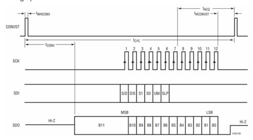
Figure 5-18 LTC2308 Timing with a Short CONVST Pulse
