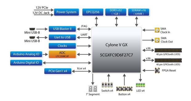
Figure 2-3 Block diagram of C5P board
