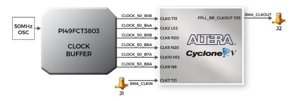
Figure 3-10 Block diagram of the clock distribution on C5P
