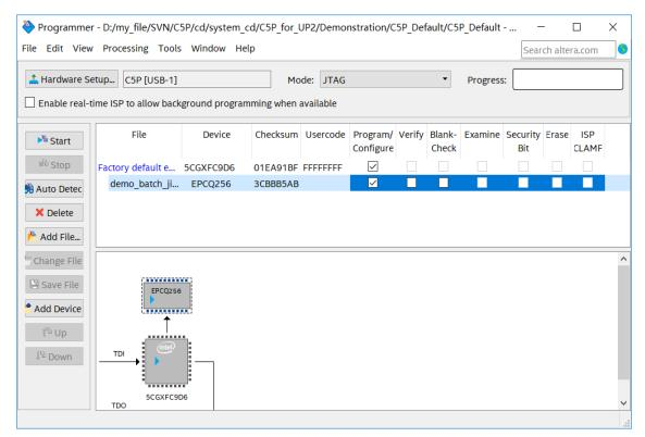
Figure 6-7 Quartus Prime Programmer window with .jic file
