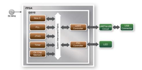
Figure 5-8 Block diagram of UART Control LED demonstration
