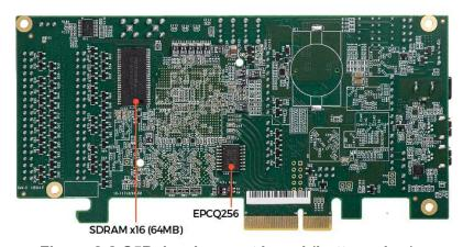
Figure 2-2 C5P development board (bottom view)
