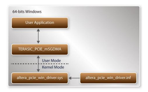
Figure 7-2 PCle Software Stack
