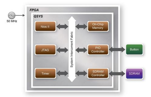
Figure 5-2 Nios II SDRAM Test System Block
