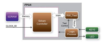
Figure 5-4 Block Diagram of Verilog SDRAM Test
