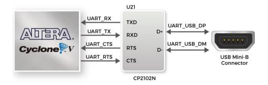
Figure 3-18 Connections between the FPGA, CP2102N chip and USB Mini-B connector
