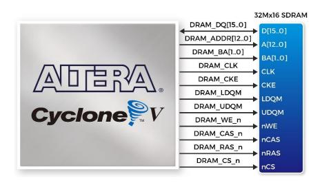
Figure 3-16 Connections between the FPGA and SDRAM
