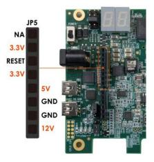
Figure 5-16 Power supply from C5P
