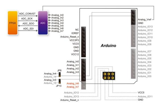
Figure 3-20 Connection and pin assignments of Arduino analog input (ADC)
