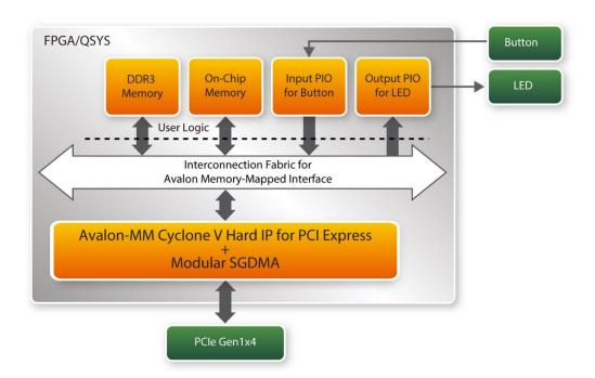
Figure 8-15 Hardware block diagram of the PCle\_DDR3 reference design
