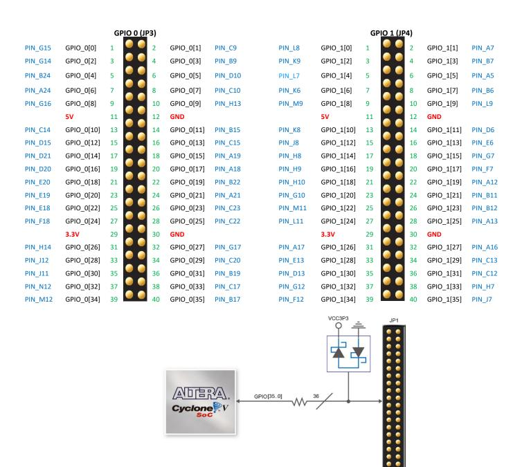
Figure 3-23 Connections between the GPIO connector and Cyclone V FPGA
