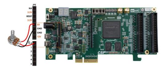
Figure 5-20 ADC Reading Demo hardware setup
