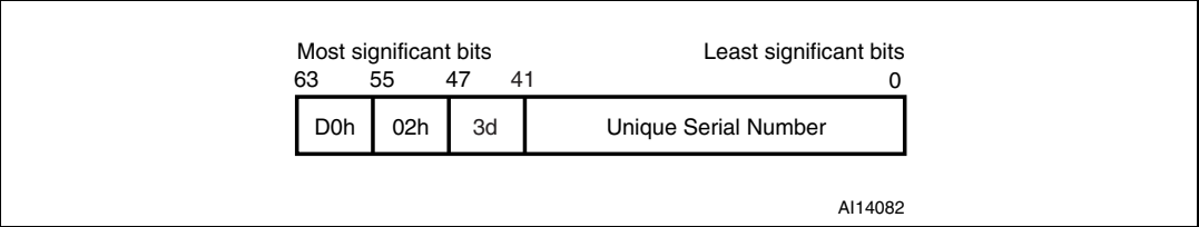
Figure 50. 64-bit unique identifier of the SRIX4K
