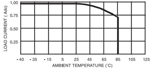
**LOAD CURRENT DERATING VS. AMBIENT TEMPERATURE**
