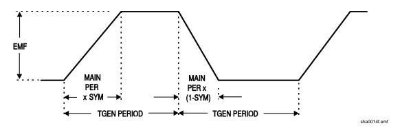
Set the main generator to 10 kHz, 10 V p-p, by pressing **FREQ**, **1**, **0**, **kHz**, and **VhiZ**, **1**, **0**, **V**; change the symmetry to 60:40 by pressing **SYM**, **6**, **0**, %; **DC OFFSET**, **0**, **V**; select **TRIANGLE**.
