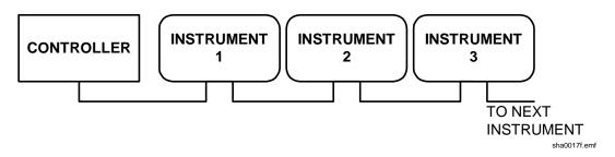
The daisy chain consists of the transmit data (TXD), receive date (RXD) and signal ground lines only. There are no control/handshake lines. This makes XON/XOFF protocol essential and allows the inter-connection between instruments to contain just 3 wires.
