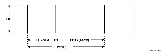
Using this technique the duty cycle range is limited to that achievable with the symmetry control (99:1). For very small duty cycles, at lower repetition rates, the triggering facilities may be used, as described in the next section.
