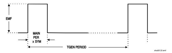
A single cycle of the main generator (i.e. a single pulse) will now be output at the default frequency of 1 kHz, so a 1000:1 duty cycle has now been achieved. Move the cursor to the TGEN period field with the **FIELD** keys and increase the period using the rotary control; although it will be difficult to see on the oscilloscope, the 1  $\mu$ s pulse width is maintained down to milliHertz repetition rates, i.e. an extremely small duty-cycle.
