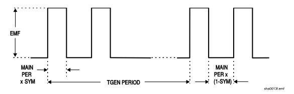
Set TGEN to 1.00 ms again (1 kHz) and the burst count to 2; this will give the waveform shown. The pulse width and interval between successive pulses is determined by the main generator frequency and symmetry; the pulse width will be PER multiplied by SYM, and the pulse low time will be PER multiplied by (1-SYM). The repetition rate of the bursts remains determined by the TGEN period.
