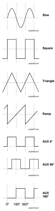
The convention adopted for phase in this instrument is illustrated in the diagram.  $0^{\circ}$  is always the first data point in waveform memory. On symmetrical waveforms  $0^{\circ}$  is the rising edge zero-crossing point for sine, square, triangle and pulse waveforms; on ramps, staircases and arbitrary waveforms  $0^{\circ}$  is always the start point.
