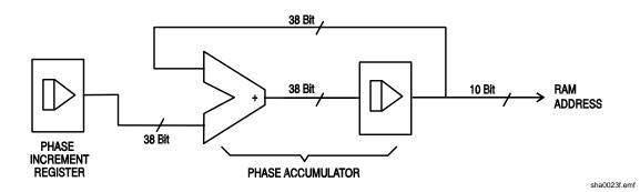
On each clock cycle the phase increment, which has been loaded into the phase increment register by the CPU, is added to the current result in the phase accumulator; the 10 most significant bits of the phase accumulator drive the RAM address lines. The output waveform frequency is now determined by the size of the phase increment at each clock. If each increment is the same size then the output frequency is constant; if it changes, the output frequency changes but with phase continuity.
