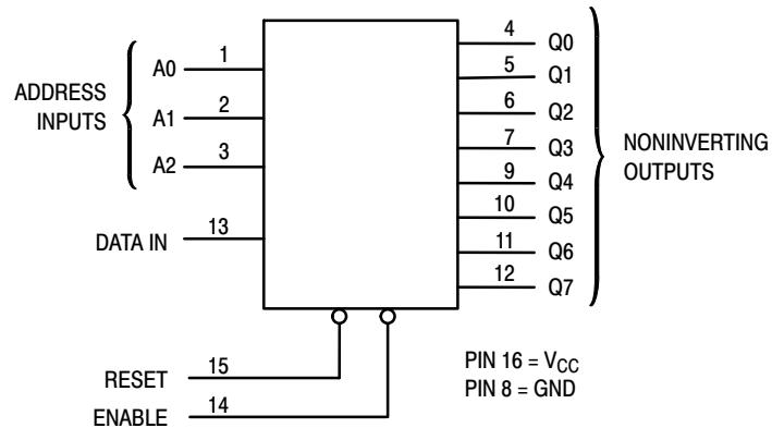
**Figure 2. Logic Diagram**
