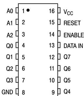
Figure 1. Pin Assignment
