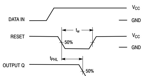
Figure 8. Switching Waveform
