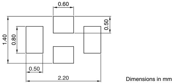
Line width be designed to match 50Ω characteristic impedance depending on PCB material and thickness.
