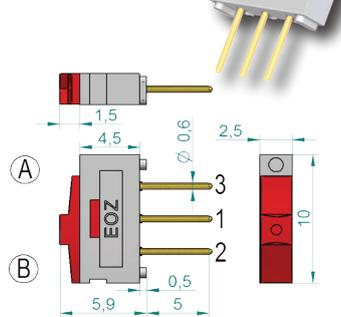
Right-angles bented pins (standard version) Red plastic slider
