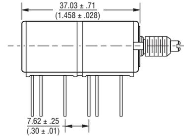
Note: The Models 83/84 dimensions for dual section assembly are for either single or dual concentric shaft styles.
