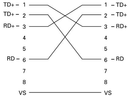
Wiring Diagram for Y-ConJack-25
