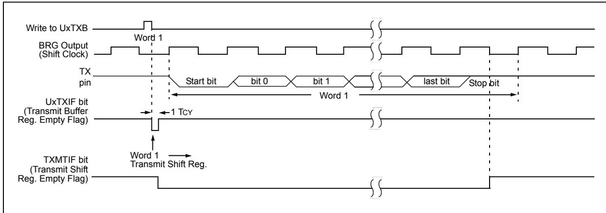
**FIGURE 31-4: ASYNCHRONOUS TRANSMISSION (BACK-TO-BACK)**
