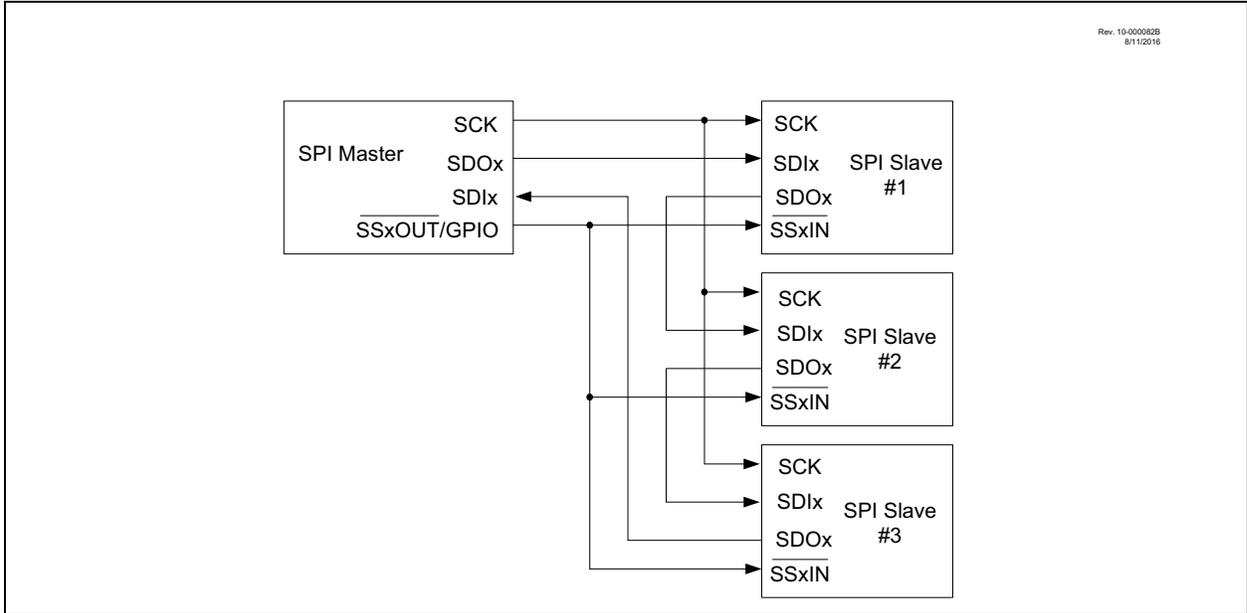
FIGURE 32-13: SPI DAISY-CHAIN CONNECTION WITH CHAINED SCK
