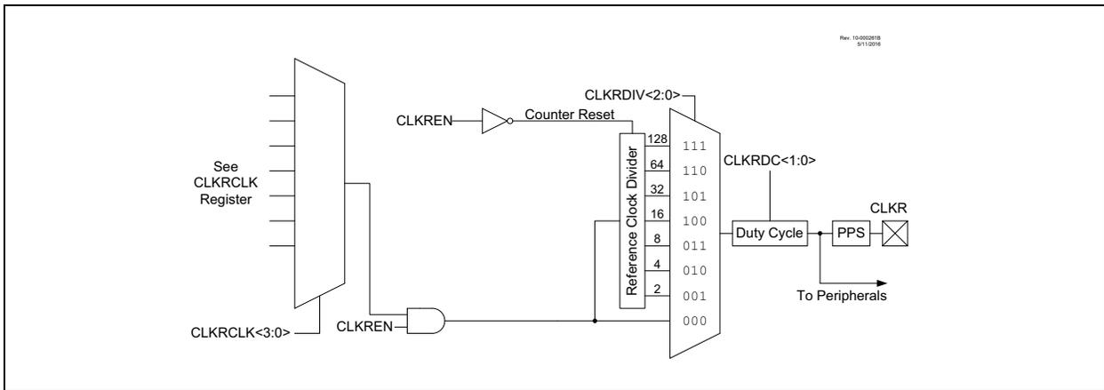
**FIGURE 8-2: CLOCK REFERENCE TIMING**
