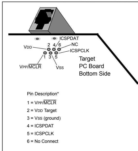
Another connector often found in use with the PICkit™ programmers is a standard 6-pin header with 0.1 inch spacing. Refer to [Figure 40-2](#).
