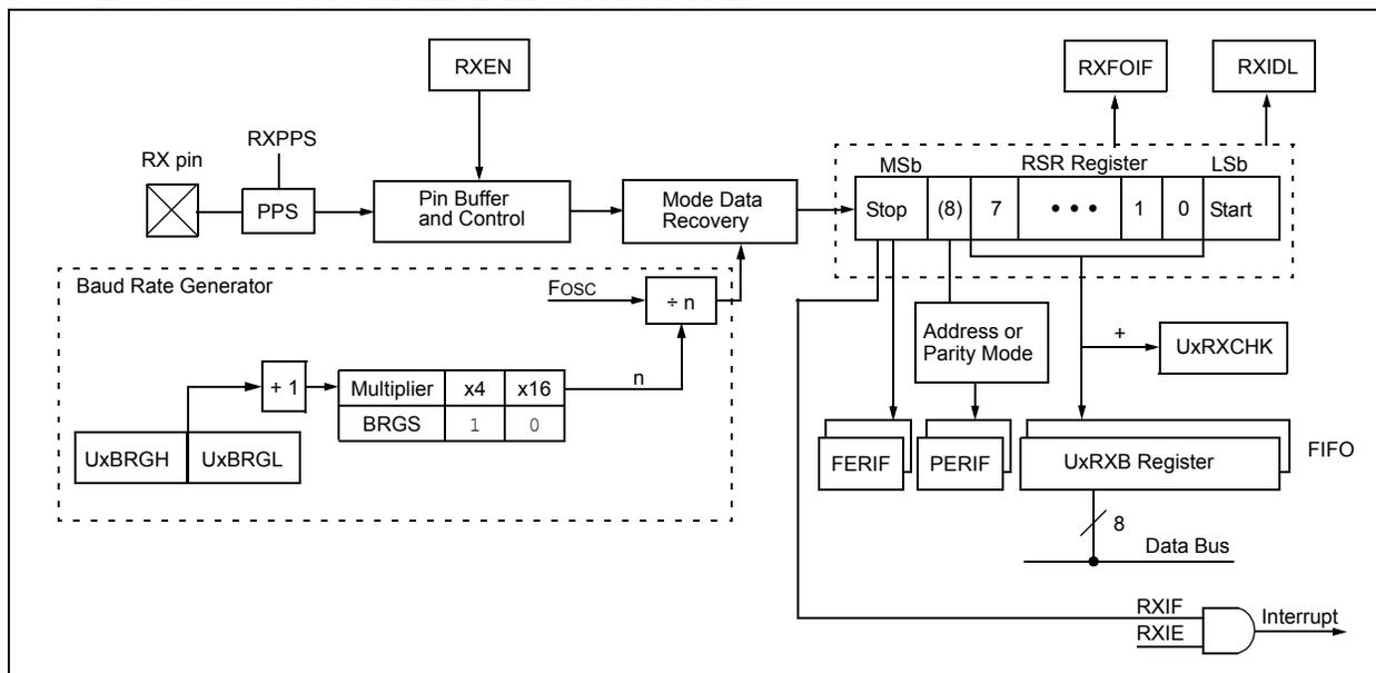
The operation of the UART module is controlled through nineteen registers:
