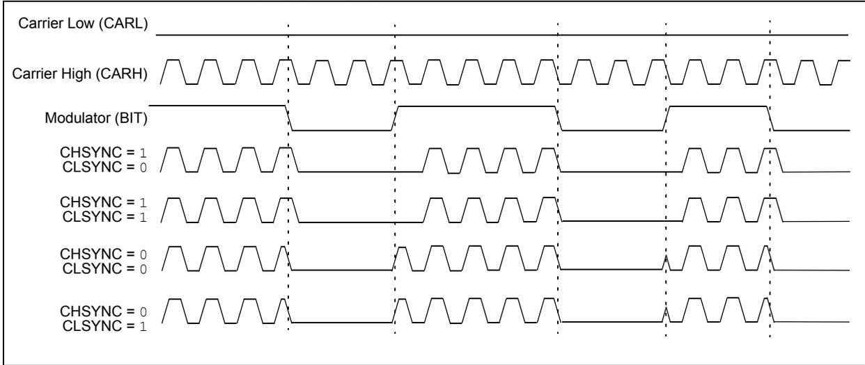
**FIGURE 30-3: No Synchronization (CHSYNC = 0, CLSYNC = 0)**
