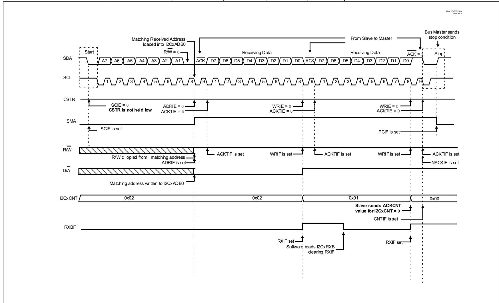
FIGURE 33-7: I<sup>2</sup>C SLAVE, 7-BIT ADDRESS, RECEPTION WITH I2CxCNT (ACKTIE = 1, ADRIE = 0, WRIE = 0)
