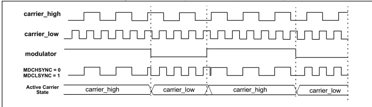
**FIGURE 30-6: Full Synchronization (CHSYNC = 1, CLSYNC = 1)**
