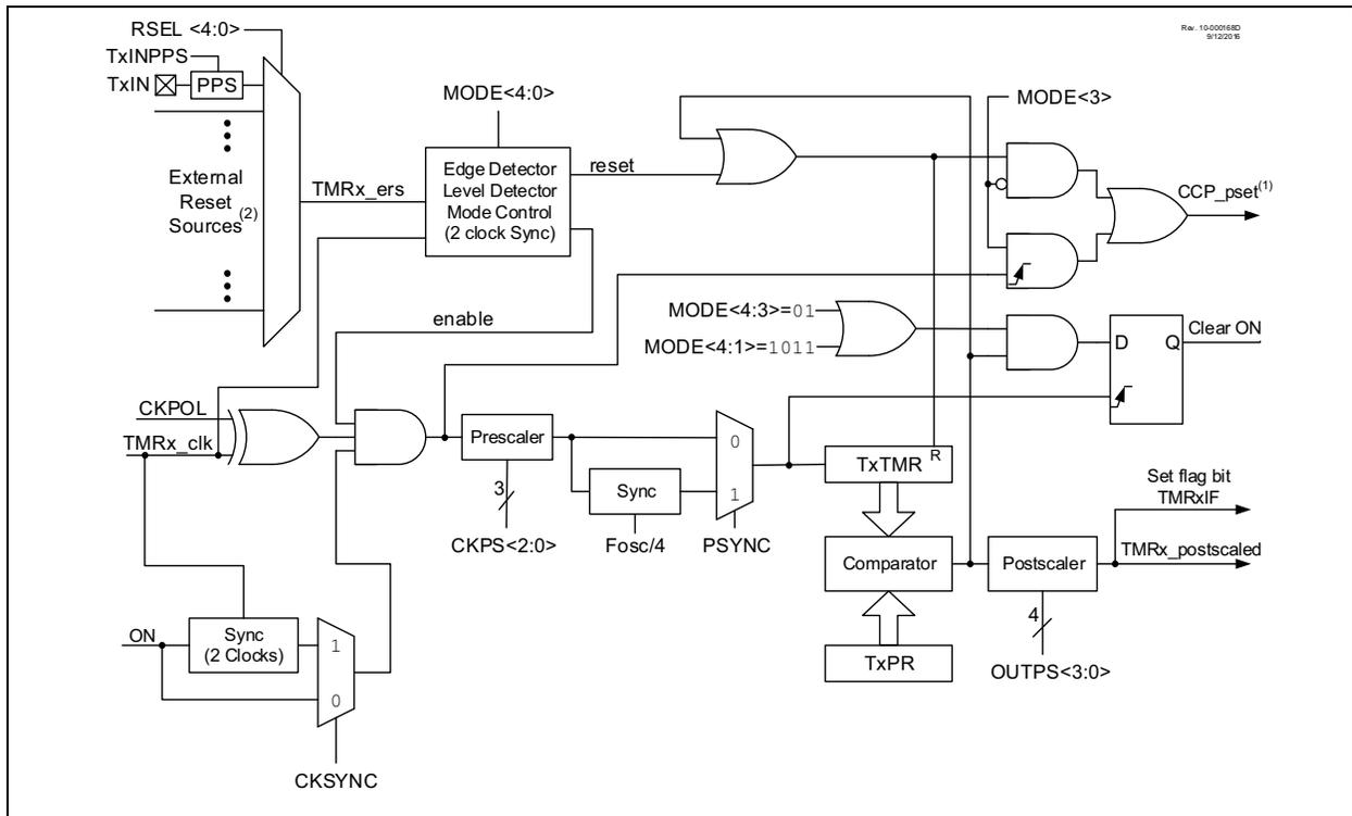
**FIGURE 22-2: TIMER2 CLOCK SOURCE BLOCK DIAGRAM**
