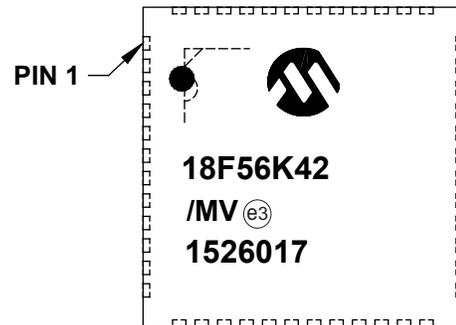
48-Lead TQFP (7x7x1 mm)
