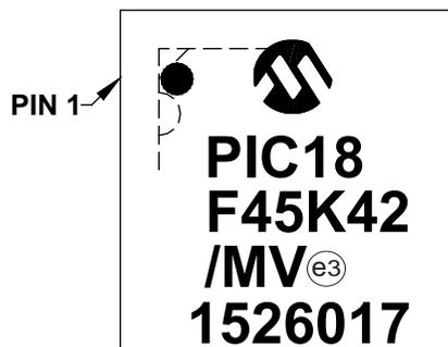
44-Lead QFN (8x8x0.9 mm)
