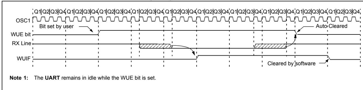
**FIGURE 31-14: AUTO-WAKE-UP BIT (WUE) TIMINGS DURING SLEEP**
