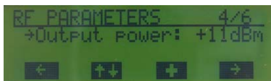
Figure 10. Menu Page: RF Parameters 4/6 (Output power is not shown in one-way receiver mode)
