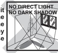
DO NOT adjust the angle of the Video Sensor Unit over 20 degrees from normal angle.
