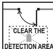
Refer to the dimensions of Detection Area for each installation height on page 5 (Fig. 1), and place the Camera unit so that the passage is fully covered by the detection area.
