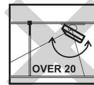
DO NOT install the Unit too close to the door so that the door intrudes the Detection Area, or the Detection Area crosses the door.
