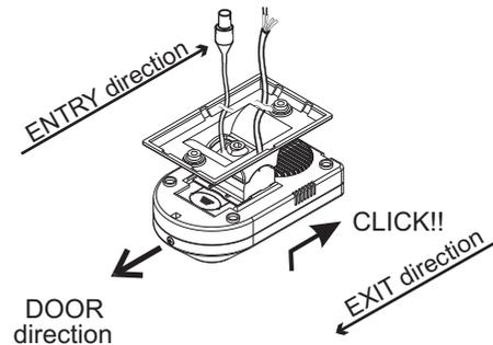
**Step 6)** Pull the wires to the Counter Display Unit and move to the Counter Display Installations stage.
