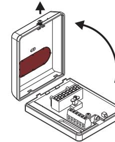
**Step 3)** Using the 6-ft. Power Cord with in-line-switch, connect the pre-stripped wires to the 12V AC 20VA transformer terminals. Strip the insulation on the opposite ends of the wires approximately 1/4 inch, and insert into the terminals on the Counter Display marked AC12V INPUT.
