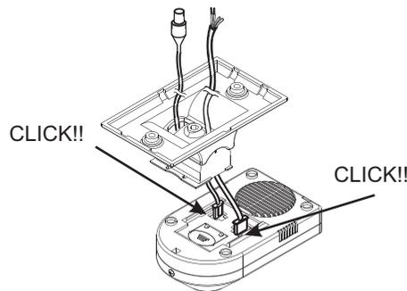
**Step 5)** Secure the Mounting Bracket and the Video Sensor Unit by sliding the unit into the guide rails of the bracket until it is secured. Make sure the round part of the Video Sensor Unit is facing the door.
