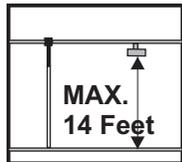
Recommend to install the Video Sensor Unit exactly in parallel with the floor so that the camera gets a birds-eye view of the Detection Area. Adjust the angle of the Unit by the maximum 20 degrees.
