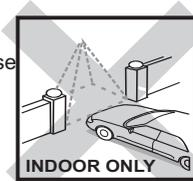
DO NOT install the video sensor unit above the floor facing directly into the sun light or other bright lights. The shadow or reflections caused by strong lights may generate false counting.
