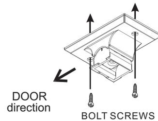
**BE CAREFUL FOR THE DIRECTION OF BRACKET INSTALLATION WHEN MOUNTING ON THE CEILING**
