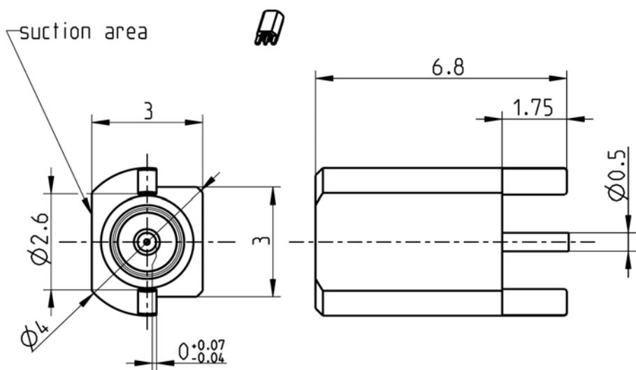
All dimensions are in mm; tolerances according to ISO 2768 m-H
