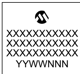
44-Lead QFN (8x8x0.9 mm)
