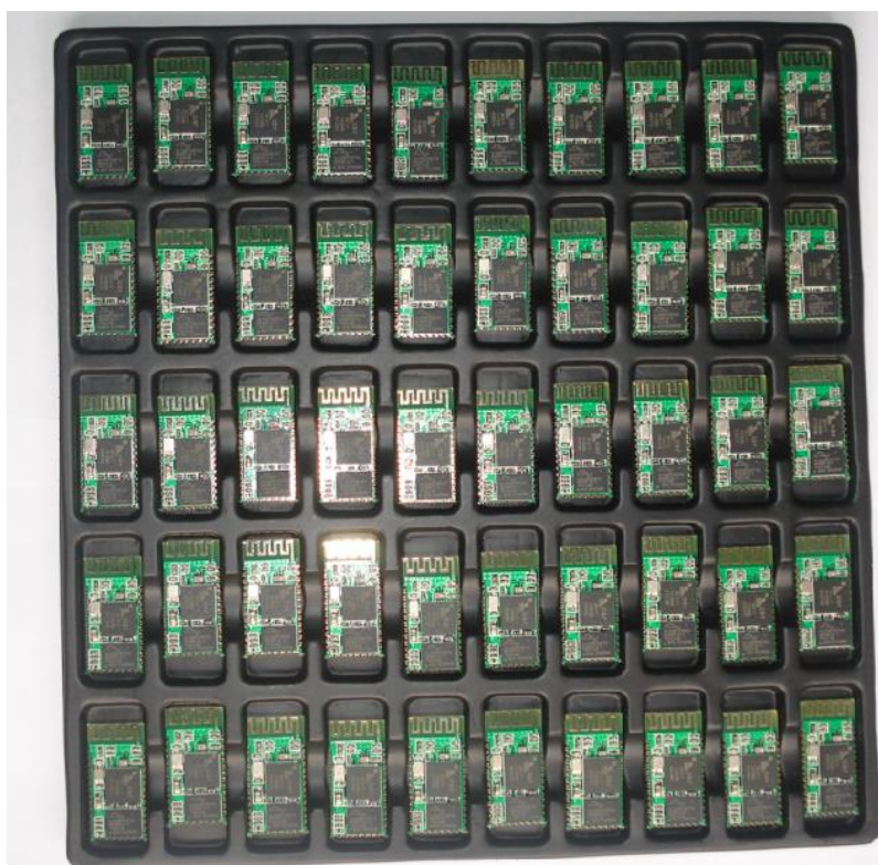
Figure 3 50 pieces chips in an anti-static blister package.
