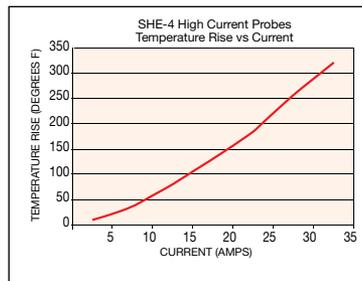
IDI current ratings are defined as the maximum current at which the temperature rise of the probe does not exceed 144°F (80°C) for a single probe in free air at ambient temperature for one hour.
