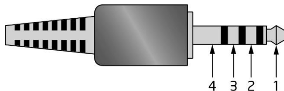
Figure 4. 4-Pin 3.5 mm (1/8 inch) Audio Jack Pin Out
