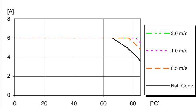
Available load current vs. ambient air temperature and airflow at  $V_1 = 12.0 \text{ V}$ ,  $V_{\text{OUT}} = 3.3 \text{ V}$ . See Thermal Consideration section.**Output Characteristics**
