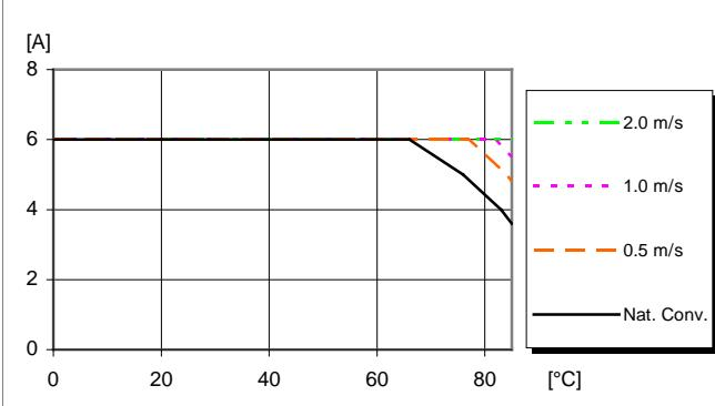
Available load current vs. ambient air temperature and airflow at  $V_1 = 12.0 \text{ V}$ ,  $V_{OUT} = 3.3 \text{ V}$ . See Thermal Consideration section.**Output Characteristics**
