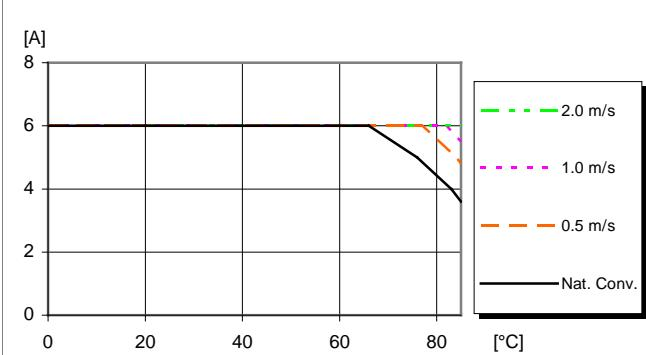
Available load current vs. ambient air temperature and airflow at  $V_i = 12.0 \text{ V}$ ,  $V_{out} = 3.3 \text{ V}$ . See Thermal Consideration section.**Output Characteristics**
