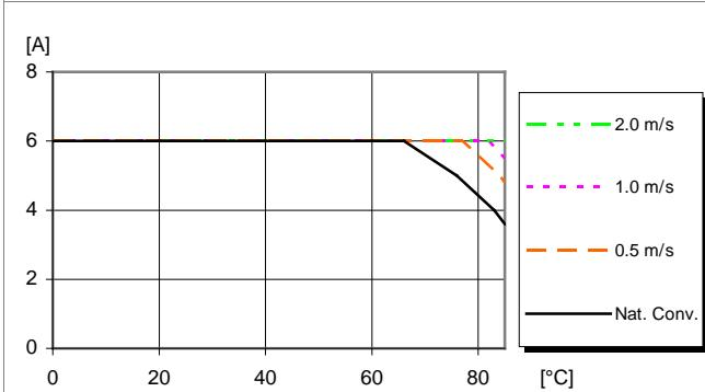
Available load current vs. ambient air temperature and airflow at  $V_1 = 12.0 \text{ V}$ ,  $V_{\text{OUT}} = 3.3 \text{ V}$ . See Thermal Consideration section.**Output Characteristics**
