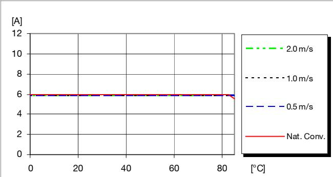
Available load current vs. ambient air temperature and airflow at  $V_i = 12.0 \text{ V}$ ,  $V_{out} = 1.8 \text{ V}$ . See Thermal Consideration section.**Output Characteristics**
