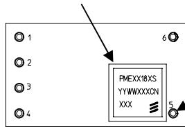
PIN 5 for measurement of minimum solder joint temperature,  $T_{PIN}$
