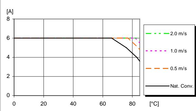
Available load current vs. ambient air temperature and airflow at  $V_i = 12.0 \text{ V}$ ,  $V_{OUT} = 3.3 \text{ V}$ . See Thermal Consideration section.**Output Characteristics**
