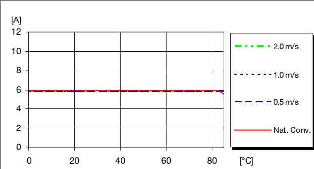
Available load current vs. ambient air temperature and airflow at  $V_1 = 12.0 \text{ V}$ ,  $V_{OUT} = 1.8 \text{ V}$ . See Thermal Consideration section.**Output Characteristics**
