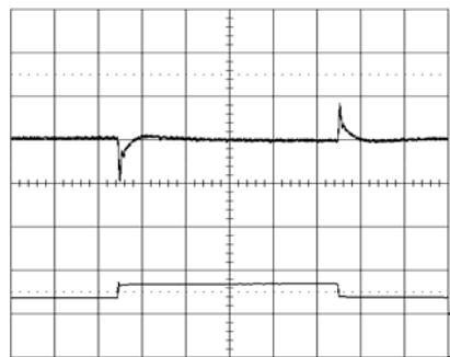
Output voltage response to load current step- change (3-6-3 A) at:
