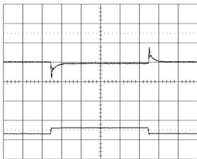
Output voltage response to load current step-change (3-6-3 A) at:
