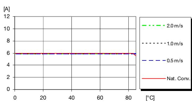
Available load current vs. ambient air temperature and airflow at  $V_i = 12.0 \text{ V}$ ,  $V_{\text{OUT}} = 1.8 \text{ V}$ . See Thermal Consideration section.**Output Characteristics**
