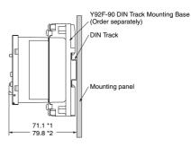
Using a PFP-50N or PFP-100N Mounting Track.
