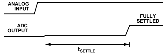
Figure 57. Step Input with Single Cycle Settling
