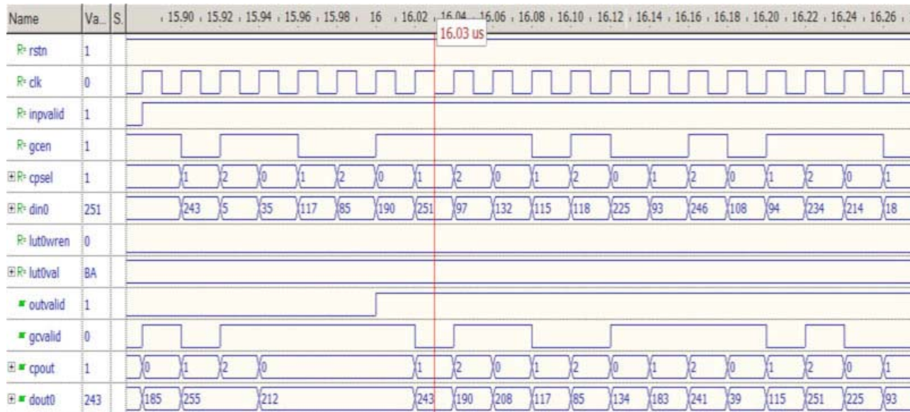
Figure 2-8. Functionality of Constant Gamma Value (= 2.2)
