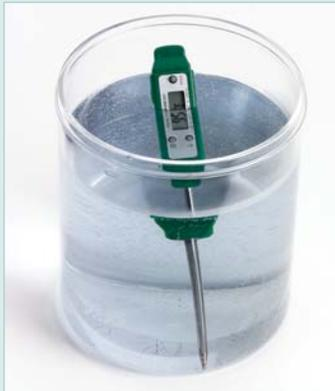
Waterproof housing allows meter to be completely submerged in water
