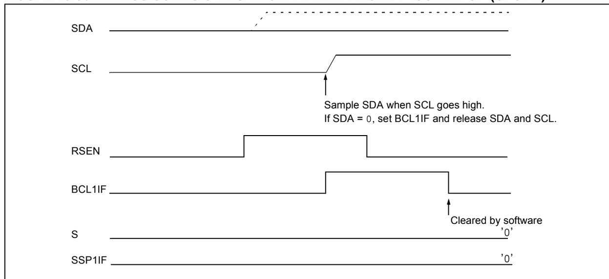
**FIGURE 25-37: BUS COLLISION DURING REPEATED START CONDITION (CASE 2)**
