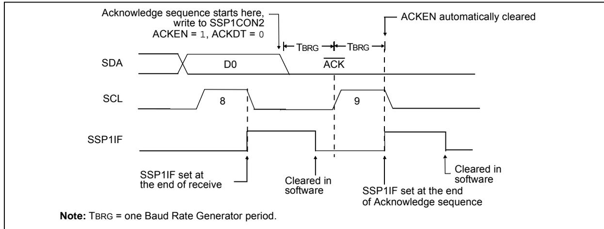
**FIGURE 25-31: STOP CONDITION RECEIVE OR TRANSMIT MODE**
