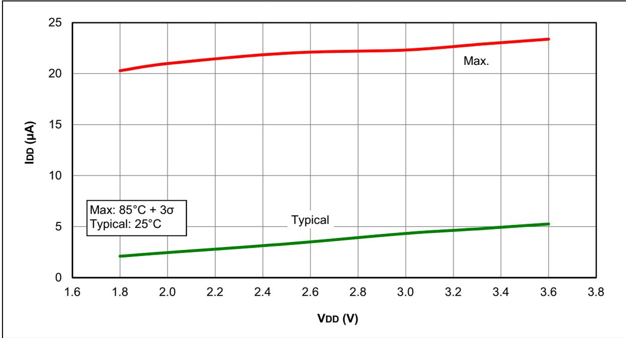
FIGURE 31-20: I<sub>DD</sub>, LFINTOSC MODE (F<sub>osc</sub> = 32 kHz), PIC12F1822 AND PIC16F1823 ONLY
