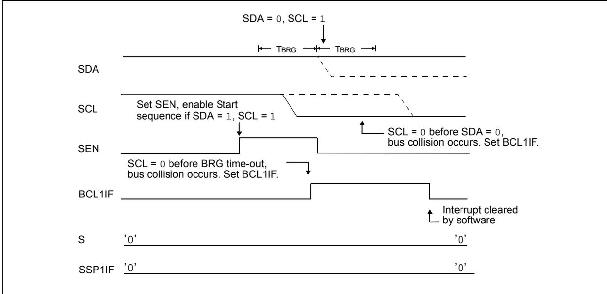
**FIGURE 25-35: BRG RESET DUE TO SDA ARBITRATION DURING START CONDITION**
