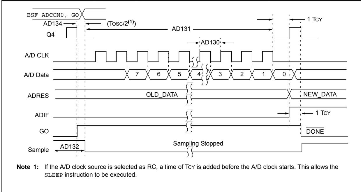
**FIGURE 30-13: PIC12(L)F1822/16(L)F1823 A/D CONVERSION TIMING (SLEEP MODE)**
