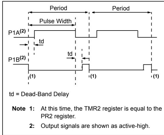
**FIGURE 24-17: EXAMPLE OF HALF-BRIDGE APPLICATIONS**
