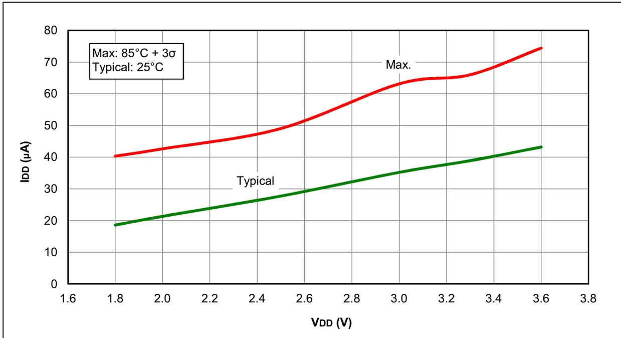
FIGURE 31-10:  $I_{DD}$ , EC OSCILLATOR, LOW-POWER MODE ( $F_{osc} = 500$  kHz),
