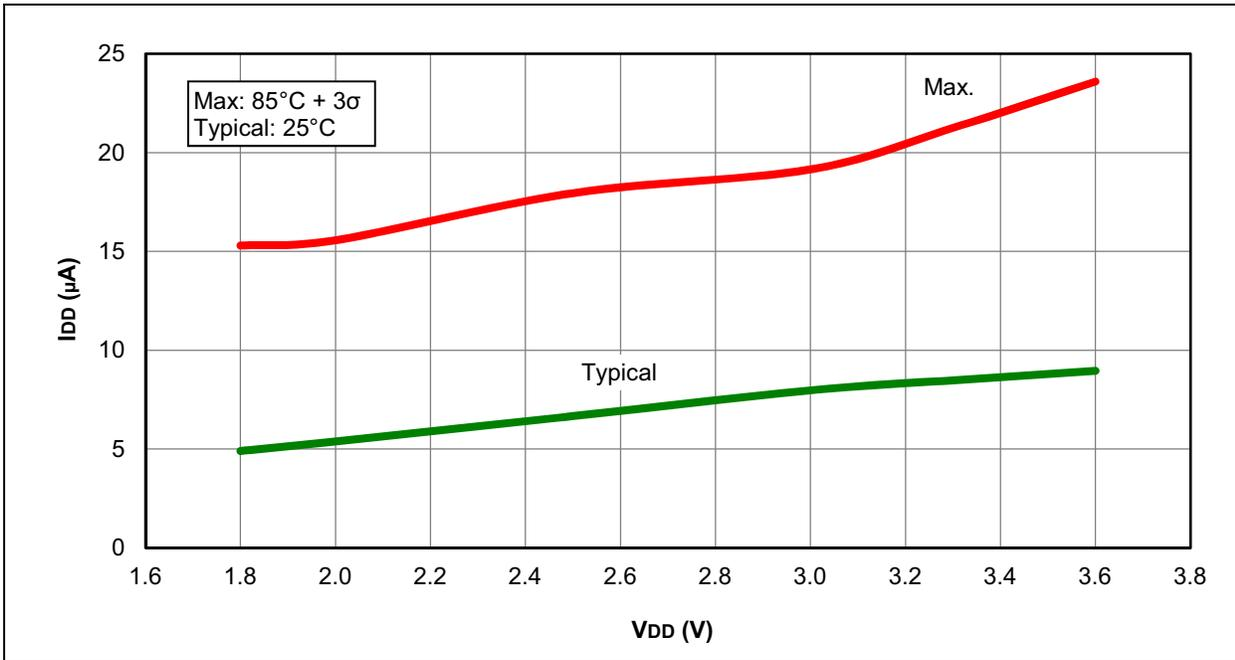
FIGURE 31-2:  $I_{DD}$ , LP OSCILLATOR MODE ( $F_{osc} = 32$  kHz),
