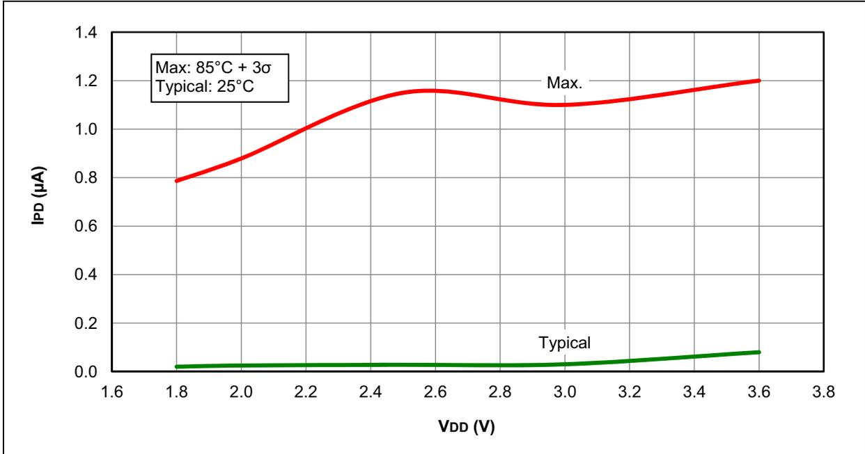
FIGURE 31-32: I<sub>PD</sub> BASE, LOW-POWER SLEEP MODE, PIC12F1822 AND PIC16F1823 ONLY
