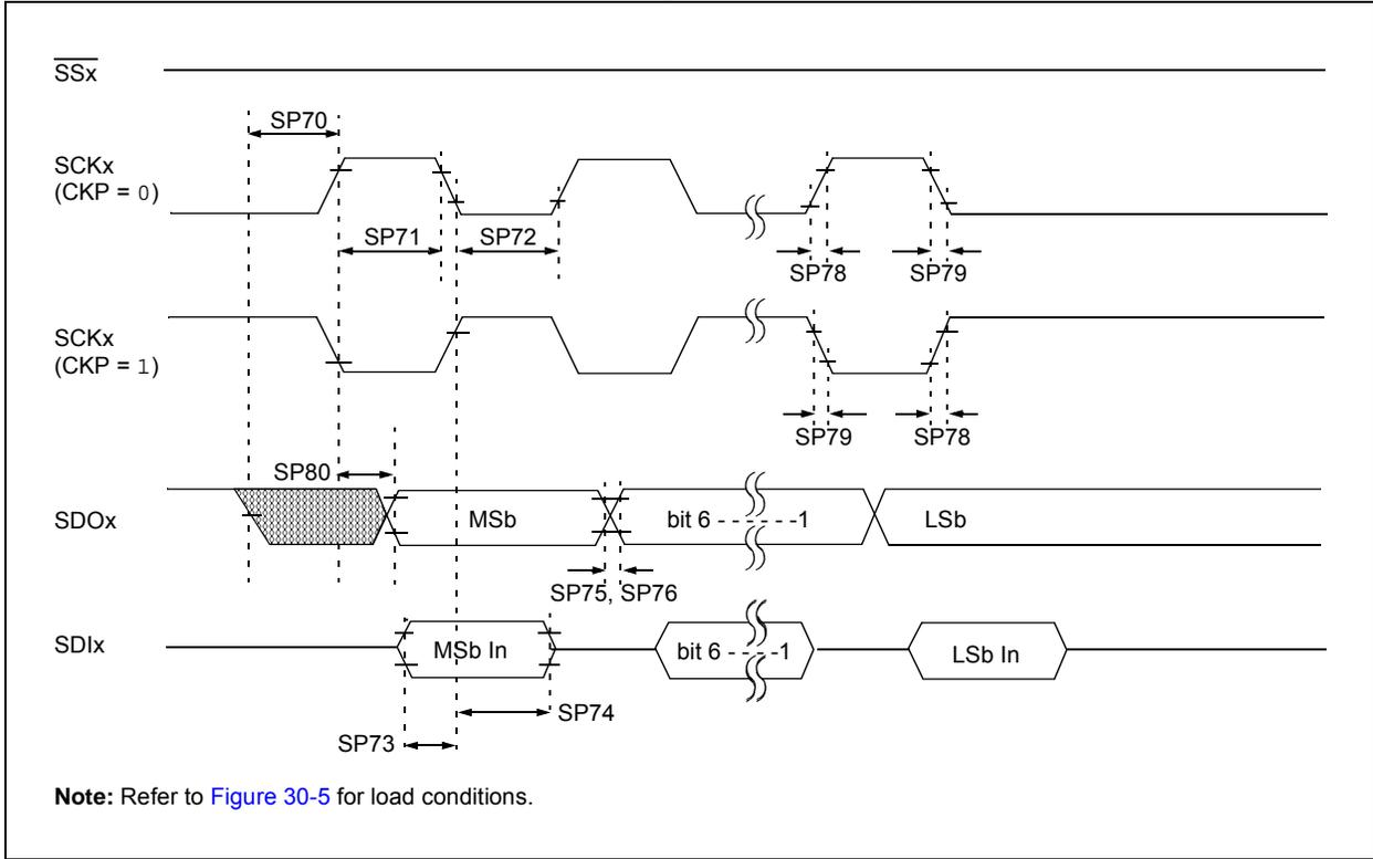
**FIGURE 30-17: SPI MASTER MODE TIMING (CKE = 1, SMP = 1)**
