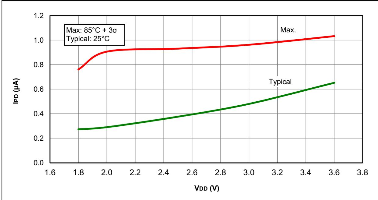
FIGURE 31-34: I<sub>PD</sub>, WATCHDOG TIMER (WDT), PIC12F1822 AND PIC16F1823 ONLY
