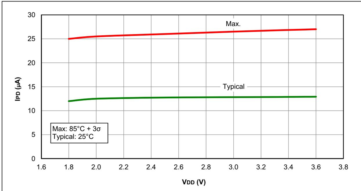
**FIGURE 31-36: IPD, FIXED VOLTAGE REFERENCE (FVR), PIC12F1822 AND PIC16F1823 ONLY**
