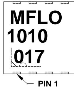
**TABLE 33-1: 8-LEAD 3x3x0.9 DFN (MF) TOP MARKING**
