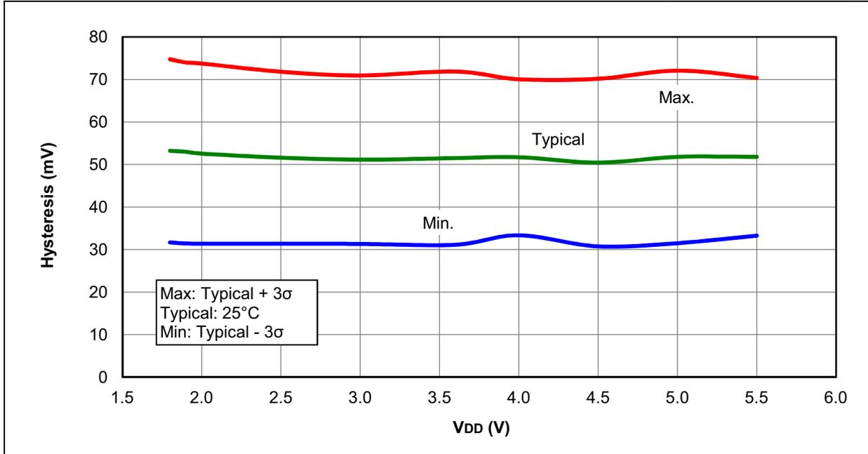
FIGURE 31-49: COMPARATOR HYSTERESIS, LOW-POWER MODE (CxSP = 0, CxHYS = 1)
