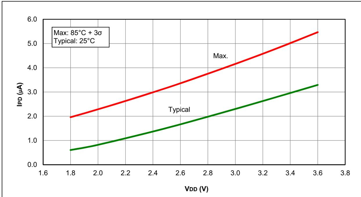
**FIGURE 31-39:** I<sub>PD</sub>, TIMER1 OSCILLATOR (F<sub>osc</sub> = 32 kHz), PIC12F1822 AND PIC16F1823 ONLY
