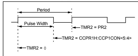
**FIGURE 24-4: SIMPLIFIED PWM BLOCK DIAGRAM**
