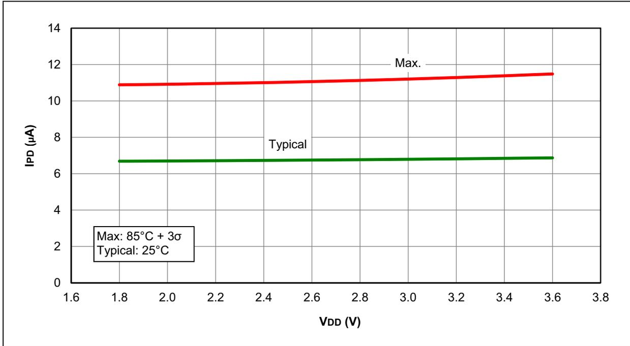
FIGURE 31-41: I<sub>PD</sub>, COMPARATOR, LOW-POWER MODE (C<sub>x</sub>SP = 0),
