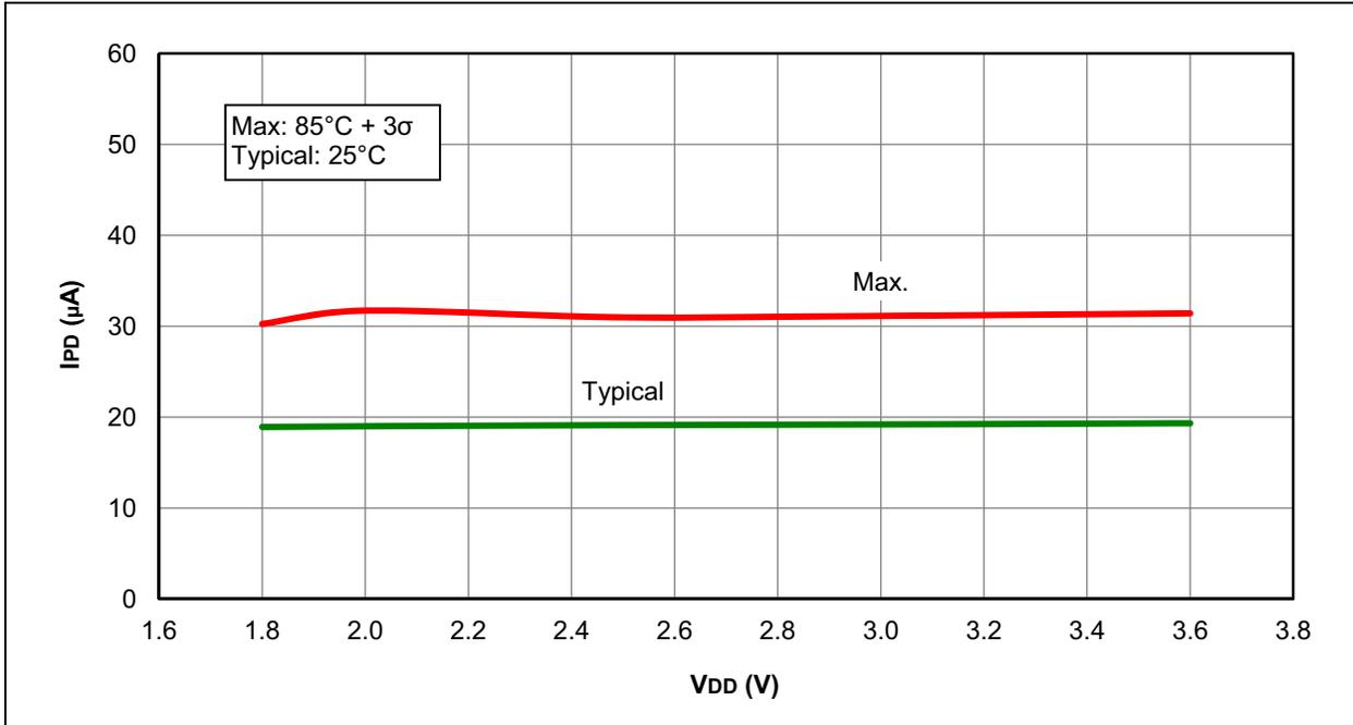
FIGURE 31-43: I<sub>PD</sub>, COMPARATOR, NORMAL-POWER MODE (C<sub>x</sub>SP = 1), PIC12F1822 AND PIC16F1823 ONLY
