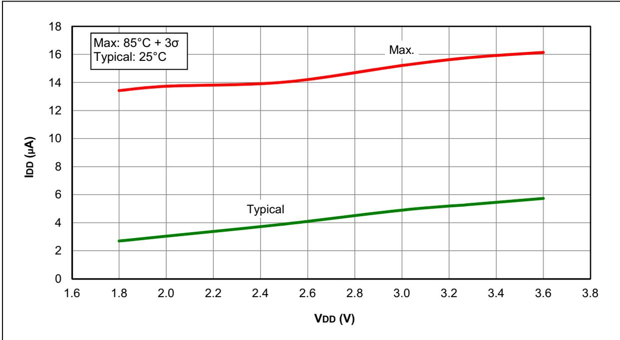
**FIGURE 31-8: I<sub>DD</sub>, EC OSCILLATOR, LOW-POWER MODE (F<sub>osc</sub> = 32 kHz), PIC12F1822 AND PIC16F1823 ONLY**
