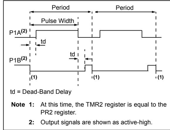
**FIGURE 24-9: EXAMPLE OF HALF-BRIDGE APPLICATIONS**
