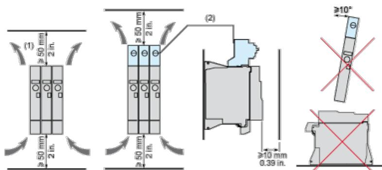
(1) Minimum value corresponding to thermal constraints.
