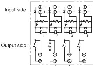
**Note1 :** Make sure that the polarity of the input terminal is correct.
