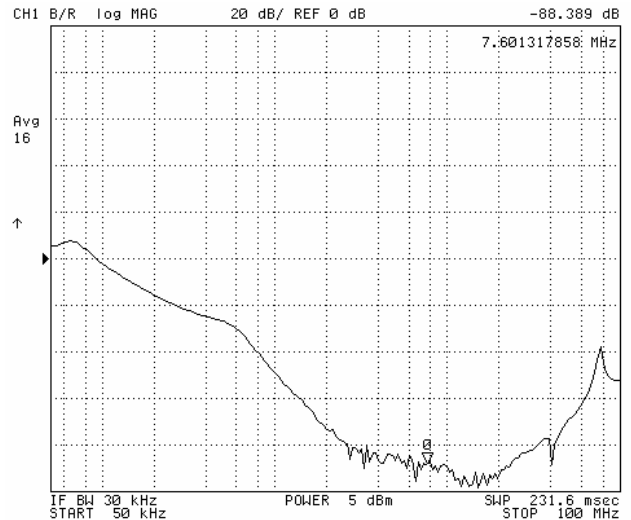
Fig. 3: Common Mode attenuation, 0.05-100 MHz. Source and load resistances are 50 Ω. Two 0.1 µF Y-caps to common line. Vertical scale: 20 dB/div, with zero dB level marked by arrow.
