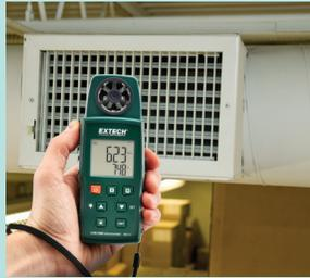
**Convenient 4-in-1 Anemometer measures Air Velocity, Air Flow, Air Temperature, and Type K Temperature. Built-in low friction ball bearing mini vane wheel for high accuracy. The Type K temperature probe function measures surface temperature up to 2372°F (1300°C). Features large dual LCD with backlighting, Data Hold, and Min/Max function.**
