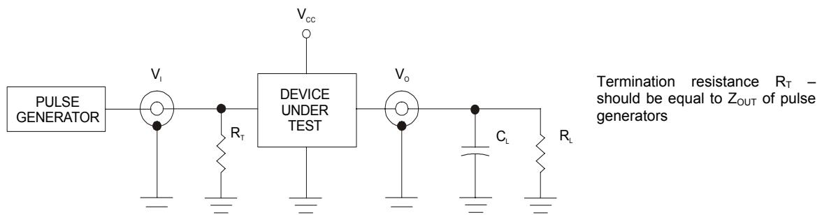
Figure 2. Test Circuit
