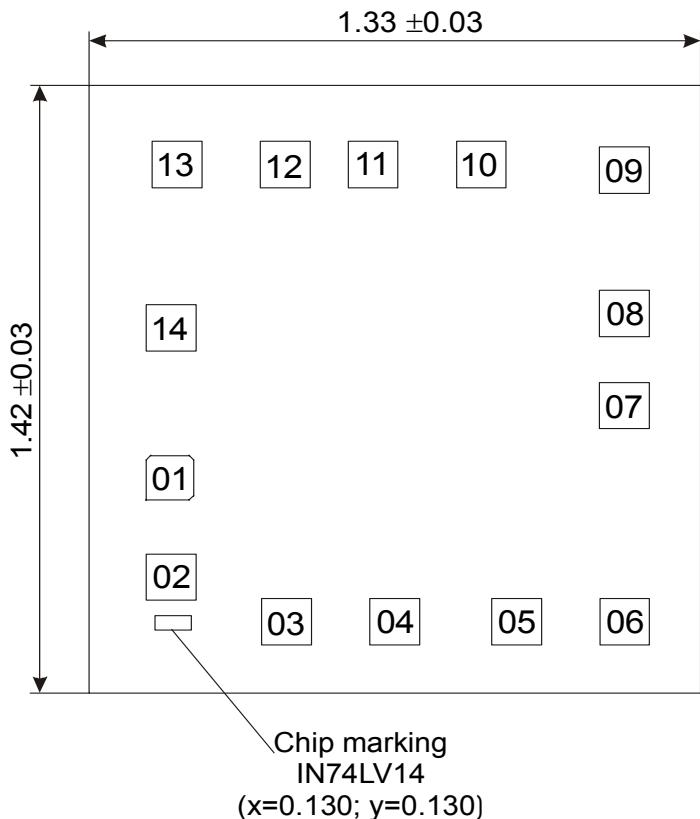
Pad size 0.108 x 0.108 mm (Pad size is given as per metallization layer)
