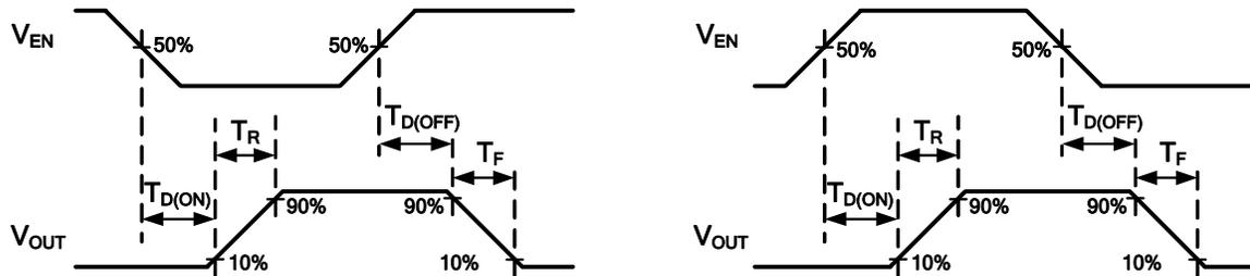
Figure 1 Voltage Waveforms: AP2501 (left), AP2511 (right)
