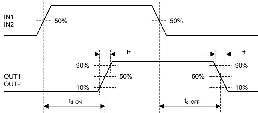
Fig1. Output Rise/Fall Time, PWM Rise/Fall Delay Time
