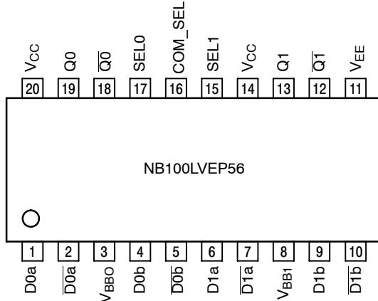
Figure 2. TSSOP-20 Lead Pinout (Top View)
