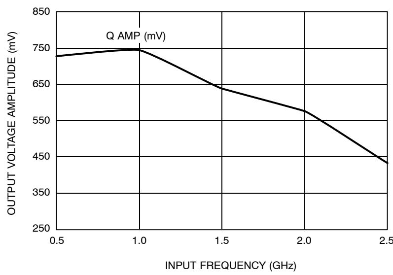
**Figure 4. Output Voltage Amplitude ( $V_{OUTPP}$ ) vs. Input Frequency ( $f_{in}$ ) at  $V_{CC} = 2.5$  V, 25°C**
