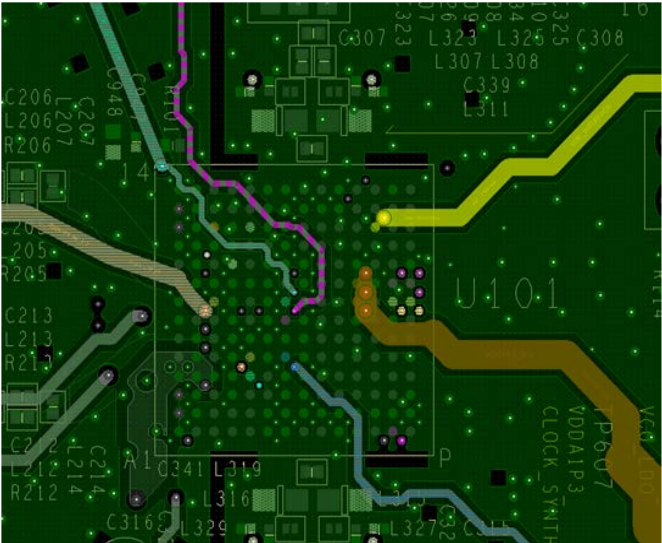
Figure 174. Layout Example of Power Supply Domains Routed with Ground Shielding (Layer 12 to Power)
