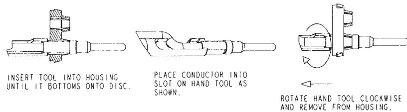
Note: Solder and PC contacts are factory assembled
