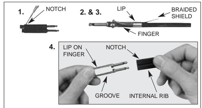
**4. ASSEMBLY:** Align grooves in fingers with internal handle ribs and insert fingers into rear of handle. Push fingers in until lips or rear of fingers snap into notches on handle.
