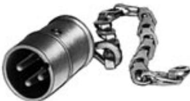
3-pin plug shorts out unused hi-Z microphone inputs or other sensitive circuits (shorting jumper installed between pins 2 and 3). 6" (152.4 mm) chain fastened to end pin to prevent plug loss. Switchcraft can install special wiring for a nominal extra charge.
