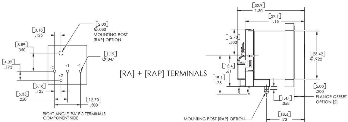
DIMENSIONS ARE FOR REFERENCE ONLY  $\frac{\text{Inch}}{\text{(mm)}}$
