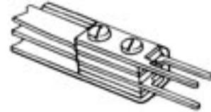
**PRINTED CIRCUIT TERMINALS** – Components can be supplied with printed circuit terminals on special order. Terminals can be specified in various lengths to accommodate different thicknesses of single and double sided boards, as well as multilayers, and flat flexible cable and circuitry.
