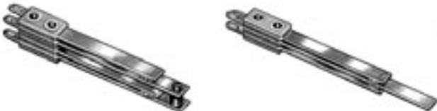
Many Tini-Stack® switching combinations are possible. Switch mounting centers are .188" (4.78 mm) (minimum). Practical spring length is 1.750" (44.45 mm) (maximum).
