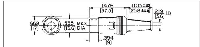
**Type 15GM7M – typical:** Male cord plug with shielded barrel and insulated snaplock plastic body. Two piece metal barrel surrounds pin insert to form an electrical shield. The entire insert assembly is held together by snapping the insulated plastic shell over the assembly. The barrel's special metal tab locks the shell in place. Standard color of plastic shell is gray. All-purpose cable clamp.
