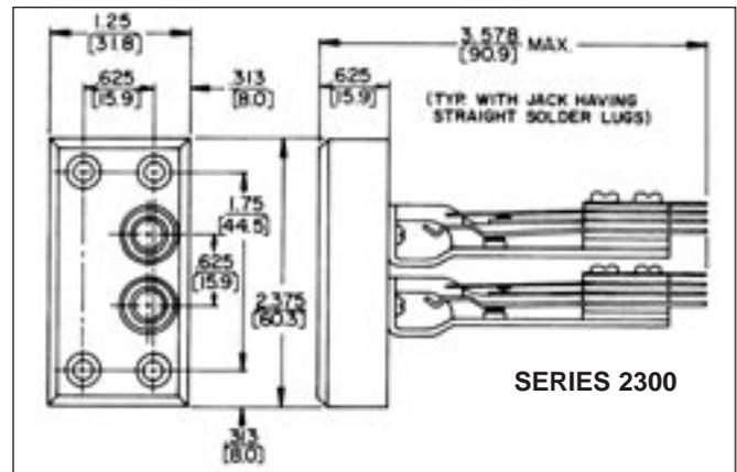
DIMENSIONS ARE FOR REFERENCE ONLY  $\frac{\text{Inch}}{\text{(mm)}}$
