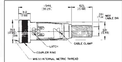
**CB-3M** 3-pin male receptacle. Housing keys insert of mating plug; bushing with external M16x1 metric thread mates with coupling ring on plug. Cup-type terminals accept wires up to #16 AWG. Mounts in .64" (16.26 mm) diameter hole from front of panels up to .125" (3.18 mm) thick, using washer and locknut supplied. Can also be "D"-hole mounted for non-turn mounting (see drawing). Pin diameter is .093".
