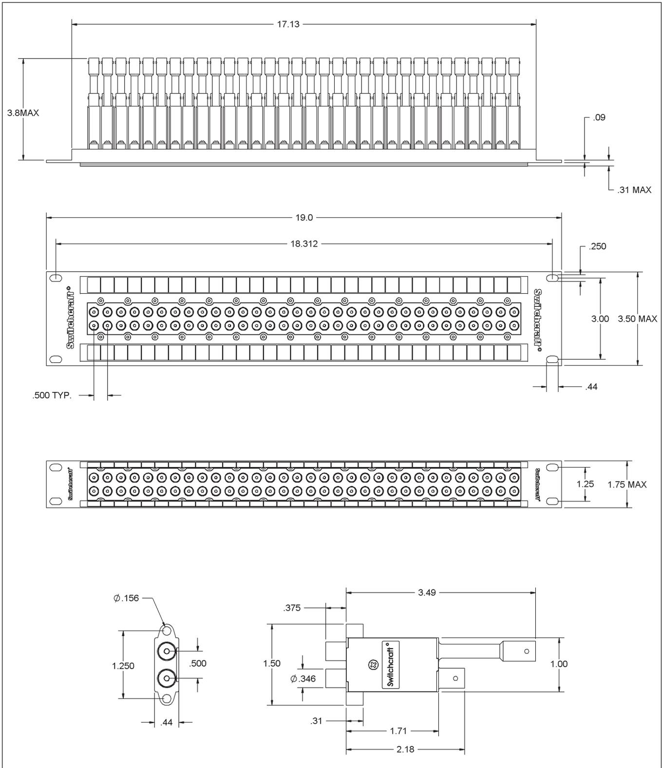
DIMENSIONS ARE FOR REFERENCE ONLY  $\frac{\text{Inch}}{\text{(mm)}}$
