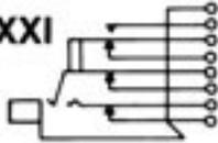
Tip closed; ring closed circuits. Isolated switching—"break" before "make" circuit.
