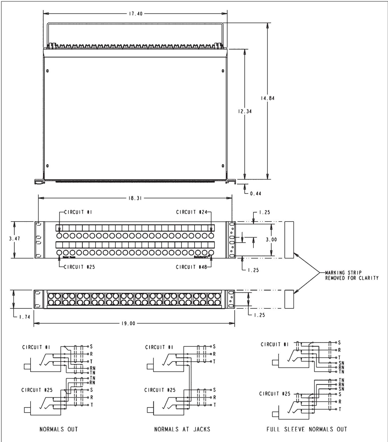
DIMENSIONS ARE FOR REFERENCE ONLY  $\frac{\text{Inch}}{(\text{mm})}$
