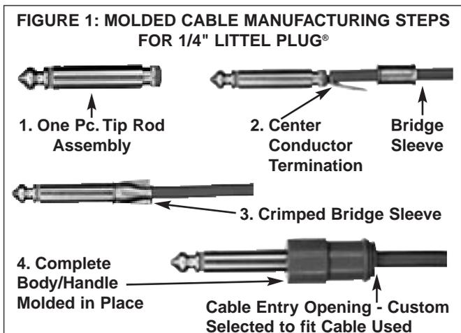
DIMENSIONS ARE FOR REFERENCE ONLY  $\frac{\text{Inch}}{(\text{mm})}$
