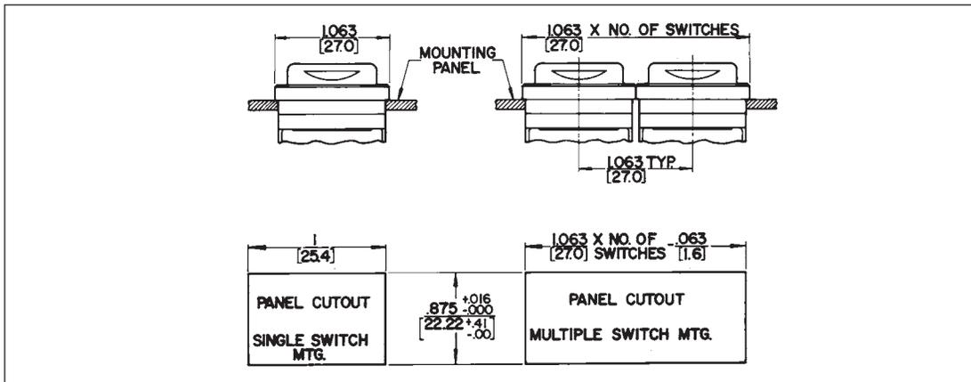
NOTE: PANEL OPENINGS FORM MULTIPLE ROW SWITCH MOUNTING
