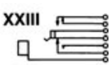
Single closed circuit plus "make" before "break". Isolated switching—"make" before "break" circuit. (J8-1D).
