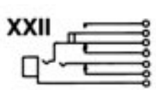
Double closed circuit. Isolated switching "make" circuit on ring spring. (J7-1A).
