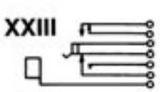
Single closed circuit plus "make" before "break". Isolated switching—"make" before "break" circuit. (J8-1D).
