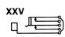
Single closed circuit. Isolated switching "break" circuit. Sleeve common to isolated switching circuit throw. (J4-1B).
