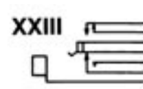
Single closed circuit plus "make" before "break". Isolated switching—"make" before "break" circuit. (J8-1D).
