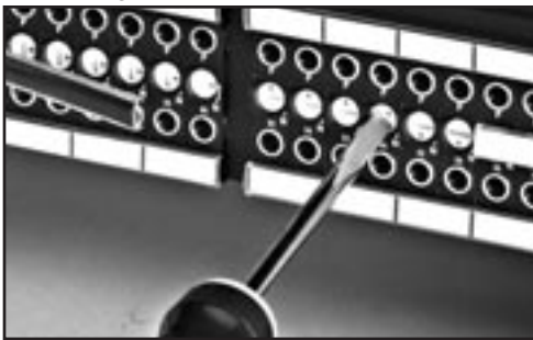
Center Strip Removes For Normaling Access
