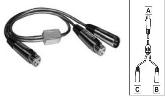
Series 391Q Y-Adapters can combine or split typical audio signals using a combination of Switchcraft Q-G<sup>®</sup> A3F and A3M cord plugs. Outputs of two microphones can conveniently be connected in parallel and connected to a single input using a 391Q23 Y-Adapter. Cabling is 2-conductor shielded, 2-foot long gray jacket with molded Y-junction at center point. Mates with Switchcraft Q-G<sup>®</sup> and QGP<sup>®</sup> connectors.
