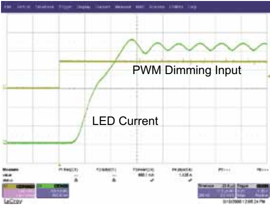
(b) PWM Dimming Rise Time Time Scale : 10µs/div
