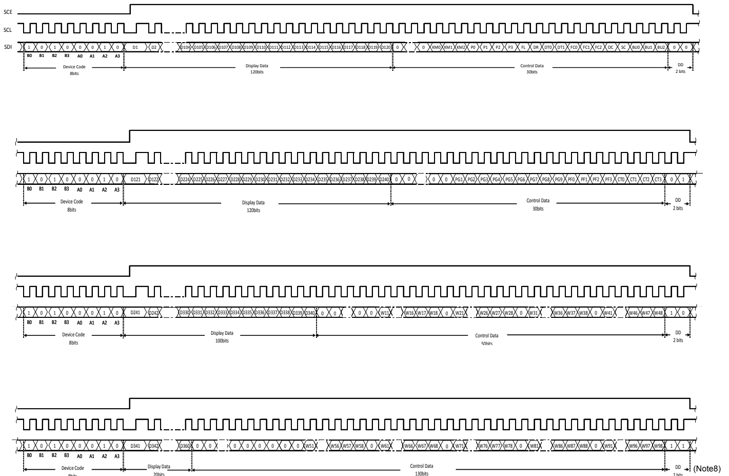
Figure 10. 3-SPI Data Transfer Format
