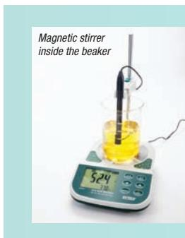
**Three models to choose from. All measure pH, mV, and Temperature. WQ510 adds Conductivity, TDS, and Salinity measurement. MQ530 has all the features of WQ510 plus it measures Dissolved Oxygen (concentration/saturation). All models have built-in Stirrer with 30, 60, and 120 minute timer or continuous. Manual store/recall 150 readings and can transfer data directly to a PC via the built-in USB interface.**
