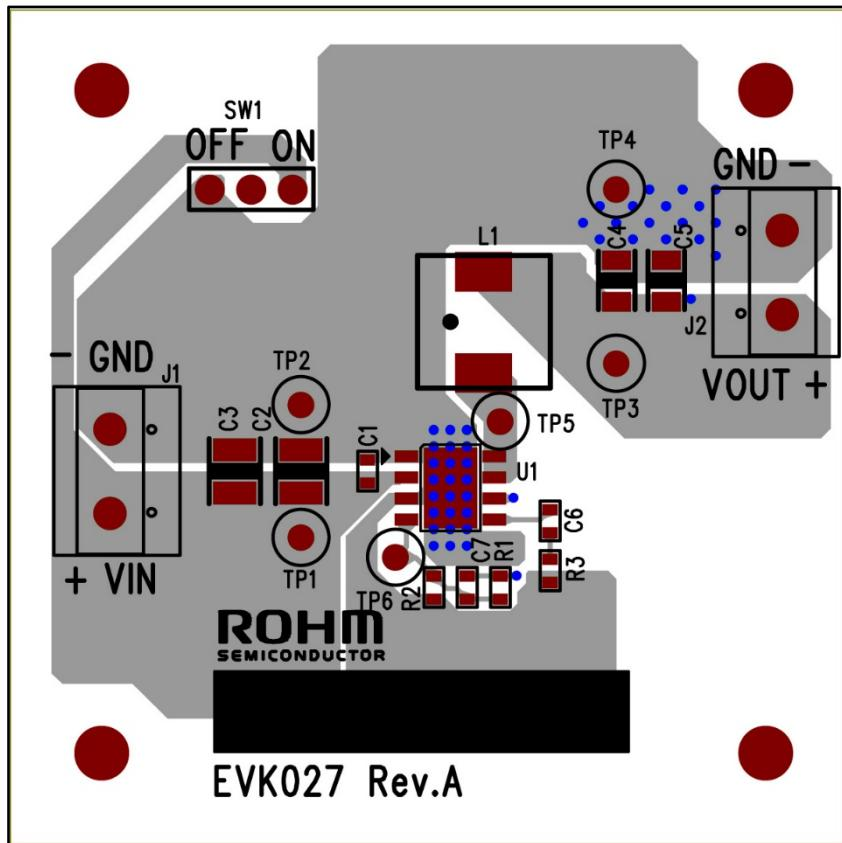
Figure 5. Top Silk Screen and Layout (Top view)
