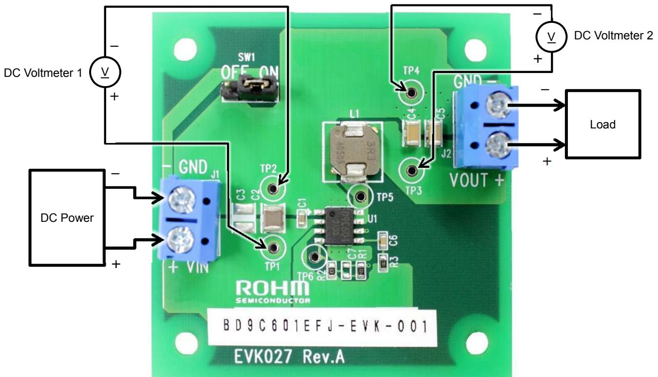
Figure 2. Connection Diagram
