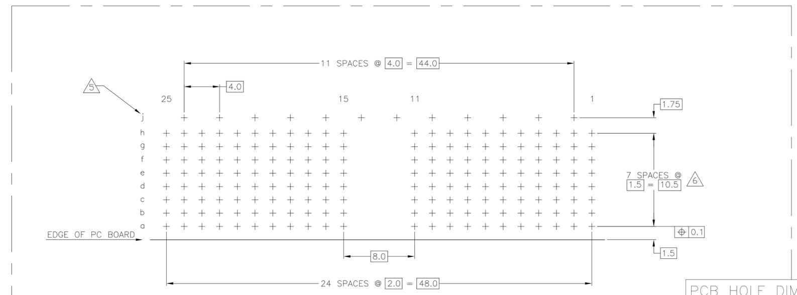
**PCB HOLE DIM ACTION PIN**
