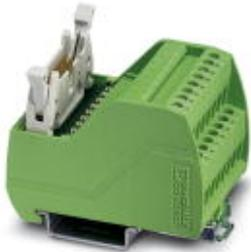
VARIOFACE module, with screw connection and flat-ribbon cable connector, for mounting on NS 35 rails, with pin strip and short and long locking latches for socket strips, 14-pos., with LED
