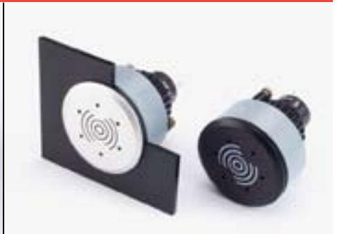
Buzzer, flush mount, 30.5mm mounting, IP40, 24VDC, 95dB ±8 at a distance of 0.1m
