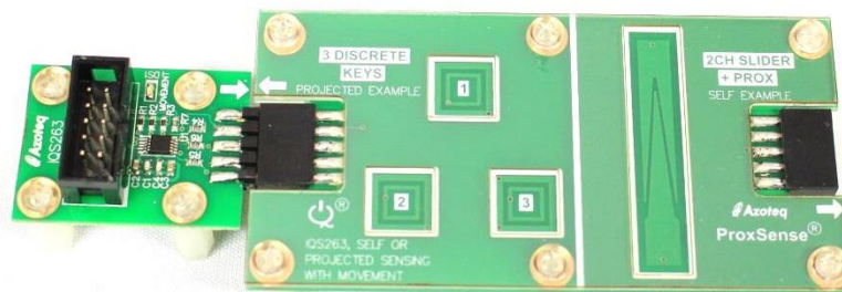
Figure 6.1 3 Keys demo board connected to driver board
