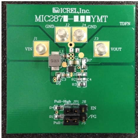
Figure 1. MIC2875-AYMT Evaluation Board
