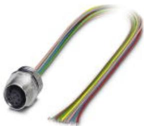
Sensor/actuator flush-type socket, 8-pos., M12, A-coded, front/screw mounting with M16 thread, with 1 m TPE litz wire, 8 x 0.25 mm<sup>2</sup>
