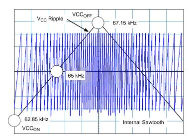
Figure 21. The V<sub>CC</sub> ripple is used to introduce a frequency jittering on the internal oscillator sawtooth. Here, a 65 kHz version was selected.
