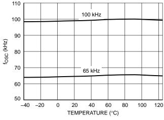
Figure 11. Frequency vs. Temperature
