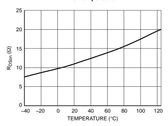
Figure 12. ON Resistance vs. Temperature, NCP1012/1013
