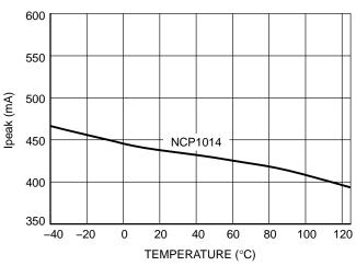
Figure 10. Ipeak-RR, V<sub>CC</sub> = 8.0 V, FB = 3.5 V vs. Temperature
