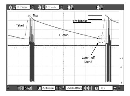
Figure 16. NCP101X Facing a Fault Condition (Vin = 150 Vdc)
