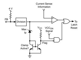
Figure 15. Simplified NCP101X Short-Circuit Detection Circuitry
