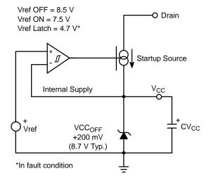
Figure 13. The Current Source Regulates V<sub>CC</sub> by Introducing a Ripple
