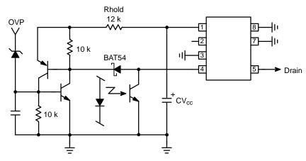
Figure 24. Two Bipolars Ensure a Total Latch-Off of the SMPS in Presence of an OVP
