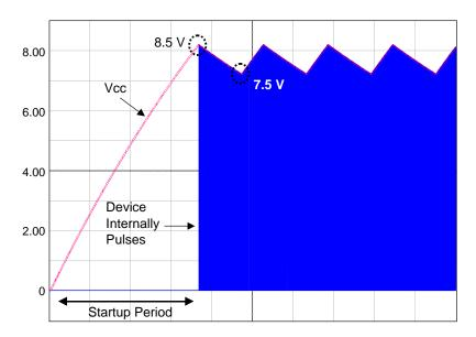
Figure 14. The Charge/Discharge Cycle Over a 10 μF V<sub>CC</sub> Capacitor
